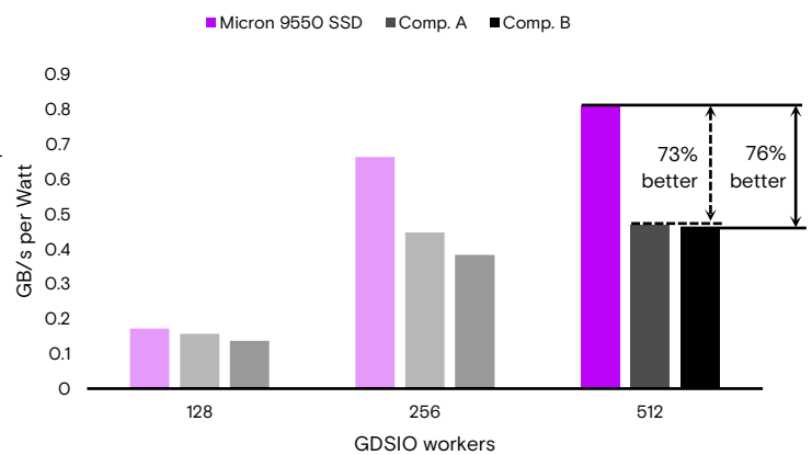
Figure 5: 4KB transfer power efficiency (GB/s per watt, higher is better)
