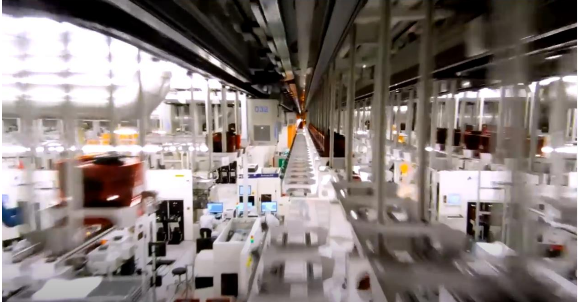
View of the fab from the ceiling, on the path of the AMHS (Automated Material Handling System)
