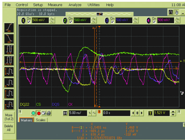
Figure 4: Examples of SI Scope Shots – One Failing, One Passing
